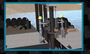
3 Using a pneumatic dispensing tool, apply epoxy to the inner face of the outer shell to bond the inner and outer shells.
